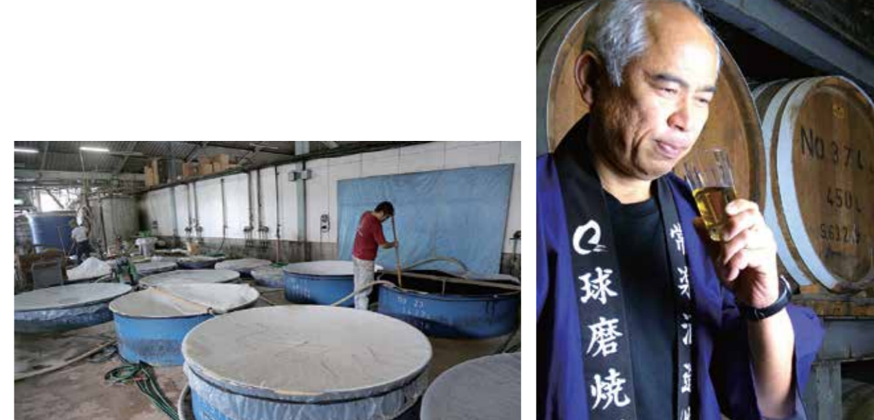
Upper left: First and second fermentations are done in enamel tanks. White, black, and yellow koji are used in different products. Upper right: Led by toji Koichi Zoza, the passionate distillery workers carefully supervise all processes, from selecting ingredients and controlling koji and mash temperatures to distillation. Left: Groundwater is used for brewing. Right: Joraku Shuzo uses atmospheric and vacuum distillation depending on the character of the shochu they wish to make.
